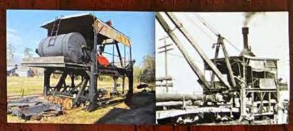
cars. At the log site, the loader lifted its wheels by resting shoes on the rail ties. Once raised, log cars could be pulled through it to load the logs. This loader is being restored by volunteers.
