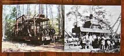
logging equipment. The skidder operated on the track and at one setting with four cables extending out, trees could be harvested from 40 acres. It was a massive machine and its operation resulted in complete destruction of vegetation on the harvest site. This is the only Clyde skidder now known to exist.
